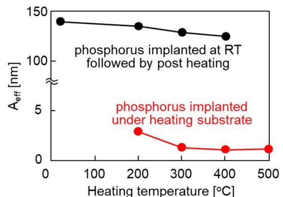
**Fig. 3**  $A_{eff}$  as a function of heating temperature during ion implantation (red solid circles) and as a function of the post-annealing temperature for implantation at RT (black solid circles)
