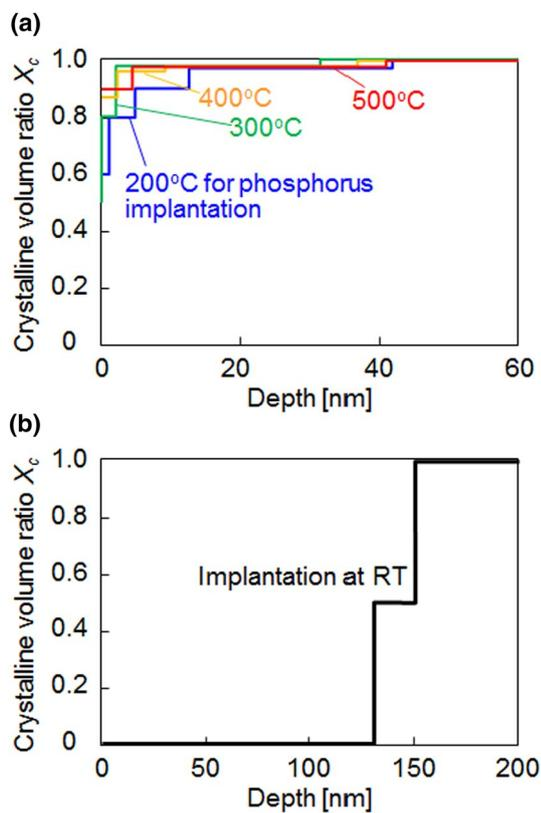
**Fig. 2** In-depth profile of  $X$  obtained by fitting calculated reflectivity spectra to experimental spectra for **a** phosphorus-implanted samples under heating ranging from 200 to 500 °C and **b** phosphorus sample implanted at RT
