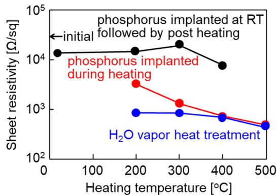
**Fig. 4** Sheet resistivity as a function of the temperature of substrate heating during phosphorus implantation for as-implanted samples (red solid circles) and samples with additional 0.9 MPa H<sub>2</sub>O vapor heat treatment at 250 °C for 3 h (blue solid circles). The sheet resistivity as a function of the post-annealing temperature for implantation at RT is also plotted by (black solid circles)
