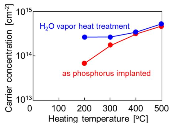
**Fig. 6** The carrier density per unit area as a function of implantation temperature for phosphorus-implanted samples (red solid circles) and samples treated in 0.9 MPa H<sub>2</sub>O vapor at 250 °C for 3 h (blue solid circles)
