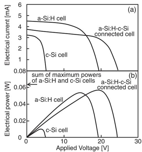
Fig. 5. (a) Solar cell characteristics and (b) electrical powers as functions of applied voltage for the a-Si:H, c-Si, and a-Si:H-c-Si connected solar cells.
