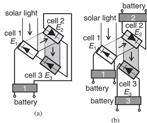
Fig. 1. Schematic images for reflection-type optic with three different solar cells, which were (a) electrically connected with electrical wires, and (b) separately connected to batteries.
