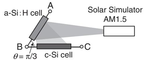
**Fig. 2.** Schematic image for reflection-type optic using a-Si:H and c-Si solar cells, which were placed facing each other with an angle of  $\pi/3$  radian and connected by electric wires.
