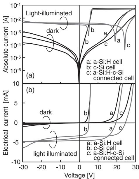
Fig. 4. (a) Logarithmic plot of absolute electrical current and (b) linear plot of electrical current as functions of applied voltages for the a-Si:H, c-Si, and a-Si:H-c-Si connected solar cells.
