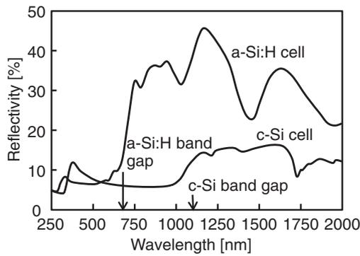
Fig. 3. Optical reflectivity spectra of the a-Si:H and c-Si solar cells.
