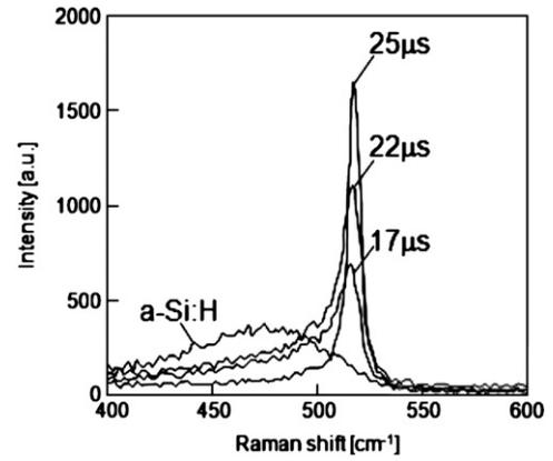
Fig. 3. Raman scattering spectra of 40-nm-thick silicon films irradiated for different dwell times ranging from 17 to 25 μs with a constant pitch in the X direction of 100 μm and a laser power of 40 W.
