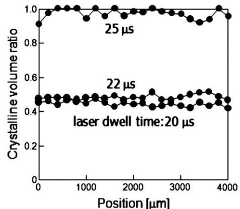
Fig. 4. CVR distribution in the normal direction of laser scanning at 40 W and with different dwell times from 20 to 25 μs.
