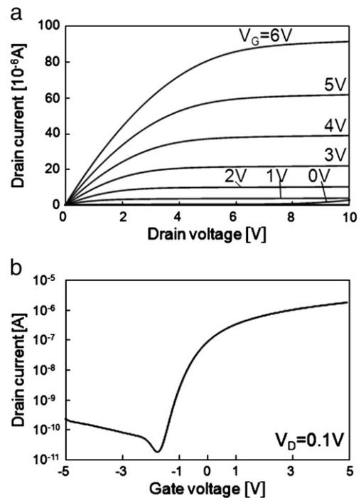
Fig. 7. Output (a) and transfer (b) characteristics of the n-channel poly-Si TFTs with a channel length and width of 100  $\mu$ m in the case of laser irradiation for 25  $\mu$ s and a laser power of 40 W.
