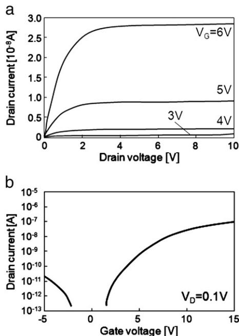
Fig. 6. Output (a) and transfer (b) characteristics of the n-channel poly-Si TFTs with a channel length and width of 100  $\mu$ m in the case of laser irradiation for 20  $\mu$ s and a laser power of 40 W.
