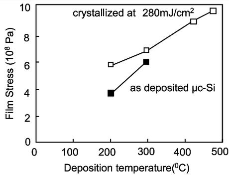
**Fig. 2** Tensile film stress as a function of deposition temperatures for as-deposited and laser-annealed samples. 50-nm-thick silicon films formed on quartz substrates at 200 and 300°C were microcrystalline and deposited by PECVD, while the films formed at temperatures above 300°C were amorphous and deposited by LPCVD
