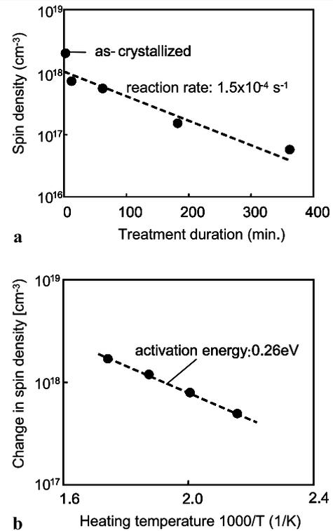
**Fig. 3** Spin density as a function of the duration of heat treatment with  $1.3 \times 10^6$  Pa  $\text{H}_2\text{O}$  vapor at 260°C for 50-nm-thick poly-Si films formed by XeCl excimer laser irradiation at an energy density of  $305 \text{ mJ/cm}^2$  (a) and spin density as a function of heating temperature for heat treatment with  $1.3 \times 10^6$  Pa  $\text{H}_2\text{O}$  vapor for 3 h (b)
