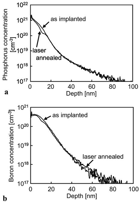
**Fig. 8** In-depth profiles of phosphorus (a) and boron atoms (b) in as-implanted and laser-annealed cases. Similar in-depth profiles were observed between the as-implanted and laser-annealed cases. Implantation with 7.5-keV  $P^+$  and 10-keV  $BF_2^+$  ions with a concentration of  $1.5 \times 10^{15} \text{ cm}^{-2}$  was carried out to silicon wafers coated with 7.9-nm thermally grown  $SiO_2$  layers
