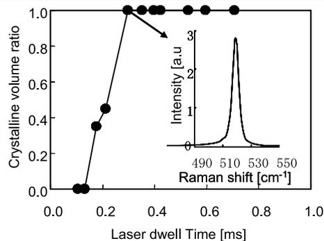
**Fig. 7** Crystalline volume ratio of 50-nm-thick silicon films formed on quartz substrates as a function of the 940-nm CW laser dwell time at a laser power intensity of  $24.7\text{ kW}/\text{cm}^2$ . The crystalline volume ratio was obtained from analysis of the optical phonon peak in Raman scattering spectra
