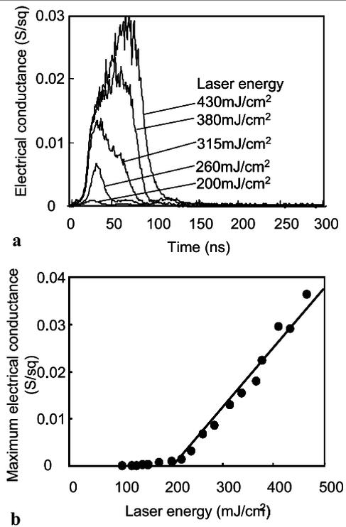
**Fig. 1** Transient electrical conductance per unit area with time for 50-nm-thick Si films (a) and the maximum electrical conductance per unit area as a function of laser energy (b). A 308-nm pulsed XeCl excimer laser with 30 ns FWHM was irradiated at 0 ns at room temperature
