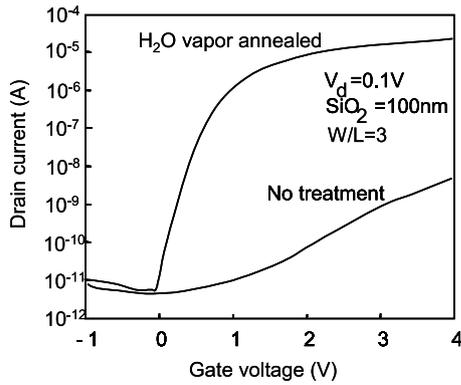
**Fig. 5** Transfer characteristics of poly-Si TFTs fabricated with no defect reduction and with heat treatment with  $1.3 \times 10^6$  Pa  $\text{H}_2\text{O}$  vapor at  $260^\circ\text{C}$  for 3 h applied after laser crystallization and TFT fabrication
