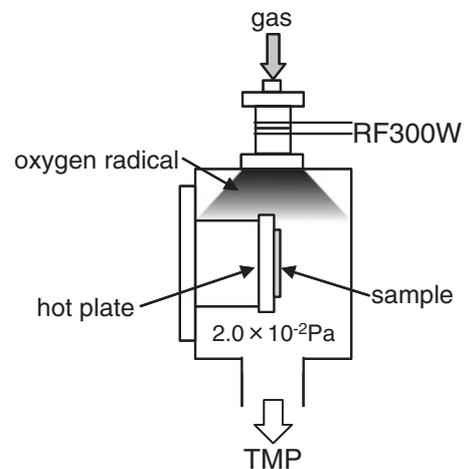
Fig. 1. Schematic apparatus of induction coupled remote plasma equipment.
