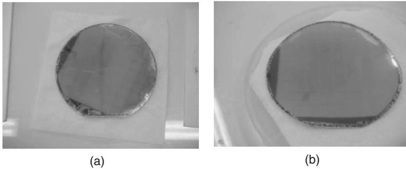
Fig. 6. Photographs of poly-Si films transferred to 4 in. plastic substrates by (a) rapid and (b) gradual coolings. The original samples had the same layer structure of plastic/silicone/epoxy/50 nm poly-Si/200 nm SiO<sub>2</sub>/1  $\mu$ m GeO<sub>2</sub>/quartz.
