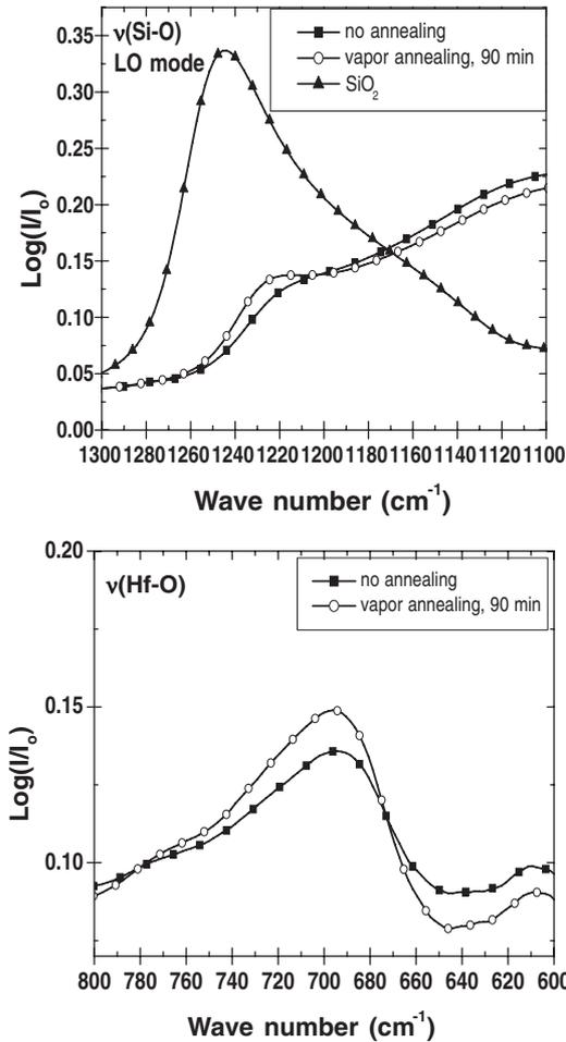
Fig. 5. FT-IR results of (a) Si-O and (b) Hf-O stretching bonds before and after H<sub>2</sub>O vapor annealing.
