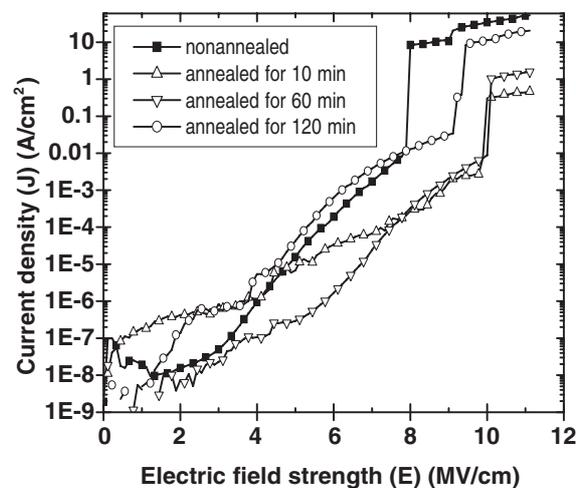
Fig. 1.  $I$ - $V$  of HfSi<sub>x</sub>O<sub>y</sub> films before and after H<sub>2</sub>O vapor annealing.
