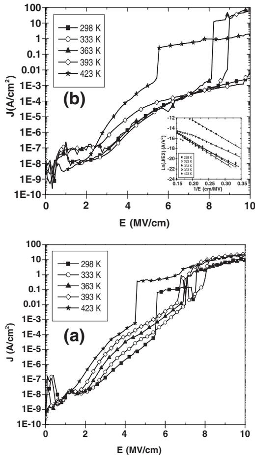
Fig. 2.  $I$ - $V$  results of samples (a) before and (b) after  $H_2O$  vapor annealing, measured at different temperatures. The inset in (b) shows the FN plots of  $HfSi_xO_y$  films after  $H_2O$  vapor annealing measured at different temperatures.
