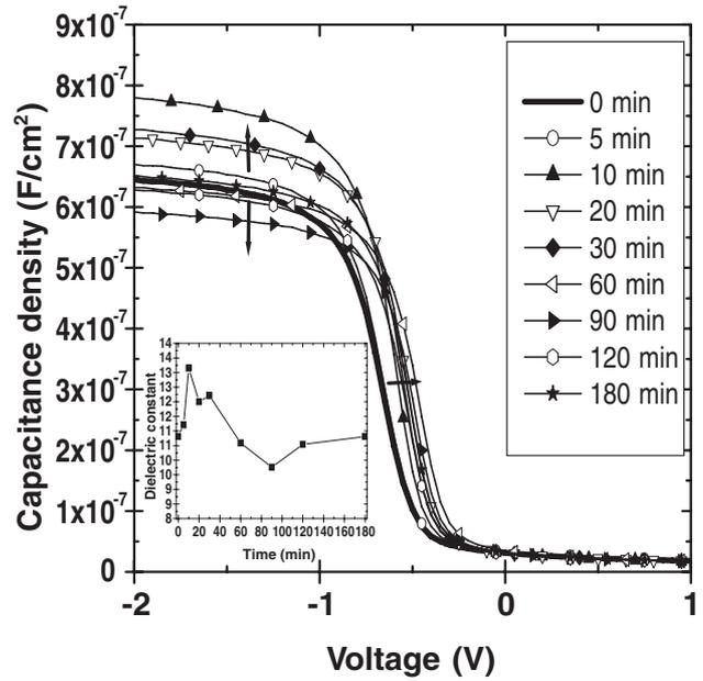
Fig. 3.  $C$ - $V$  of  $HfSi_xO_y$  films before and after  $H_2O$  vapor annealing for different times. The inset shows dielectric constants of  $HfSi_xO_y$  films for different annealing times.
