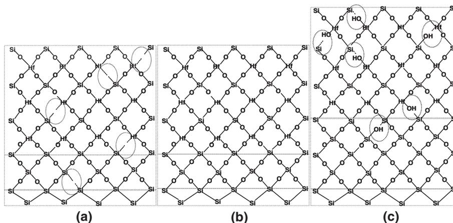
Fig. 6. Model for explaining effects of H<sub>2</sub>O vapor annealing for fixing defective bonds in bulk high- $\kappa$  HfSi<sub>x</sub>O<sub>y</sub> films. Bond structure (a) before H<sub>2</sub>O vapor annealing, (b) after short H<sub>2</sub>O vapor annealing, and (c) after more than 60 min of annealing.
