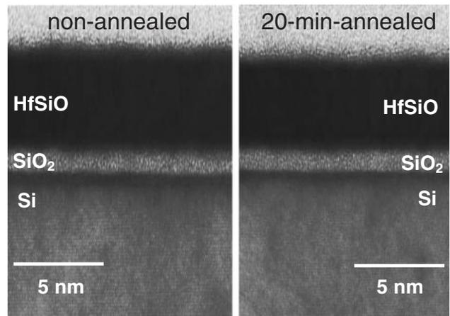
Fig. 4. TEM images of  $HfSi_xO_y$  films before and after 20 min  $H_2O$  vapor annealing.
