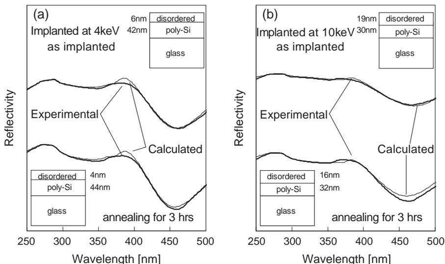
Fig. 1. Optical reflectivity spectra of ultra violet region of samples for as-implanted sample and after annealing for 3 h. (a) An energy for ion implantation is 4 keV; (b) an energy for ion implantation is 10 keV. Calculated spectra are also shown.
