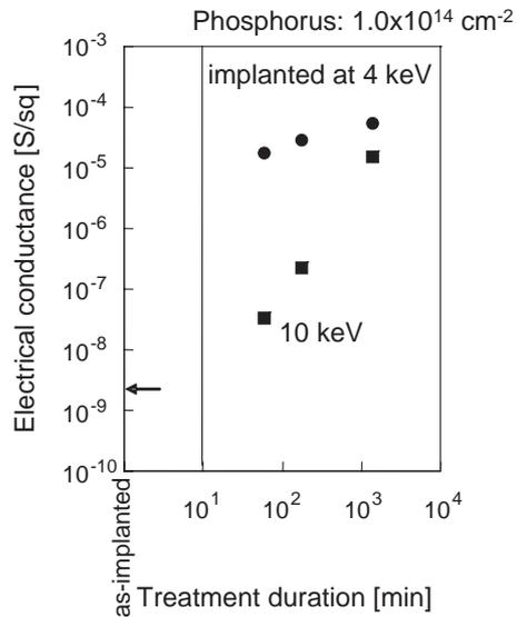
Fig. 2. Electrical conductance of phosphorus-doped silicon films implanted at 4 keV (solid circle) and 10 keV (solid square).
