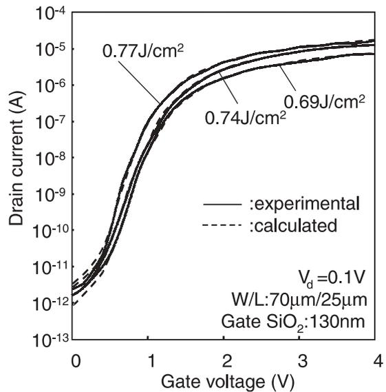
**FIGURE 3** Transfer characteristics of  $n$ -channel poly-Si TFTs fabricated at joule heating energy densities at 0.69, 0.74 and  $0.77 \text{ J/cm}^2$ , respectively (solid curve). The calculated drain current is also presented by dashed curve for each joule heating energy density (dashed curve)
