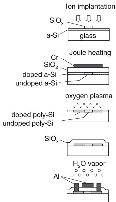
FIGURE 1 Schematic fabrication flow of poly-Si TFTs
