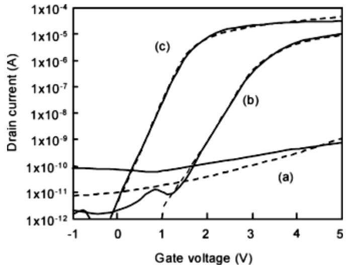
Fig. 3. Transfer characteristics for TFTs fabricated with (a) no oxygen plasma or no  $\text{H}_2\text{O}$  vapor heat treatments, (b) oxygen plasma treatment, and (c) additional  $\text{H}_2\text{O}$  vapor heat treatment. Dashed curves were calculated transfer characteristics which were obtained by a numerical calculation program.
