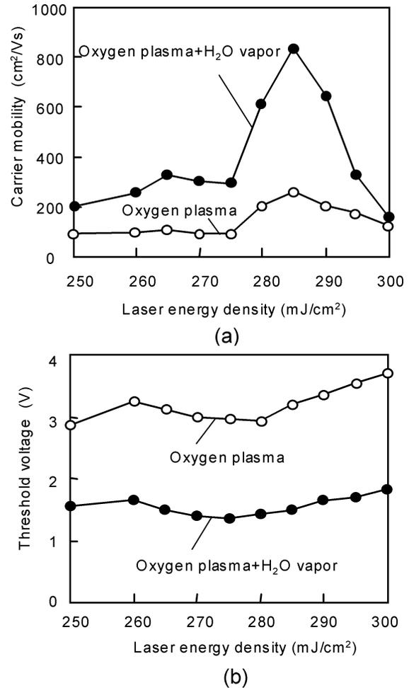
Fig. 5. (a) Effective carrier mobility and (b) threshold voltage as a function of laser energy density for TFTs fabricated with oxygen plasma treatment and combination of oxygen plasma with high-pressure H<sub>2</sub>O vapor heat treatment.
