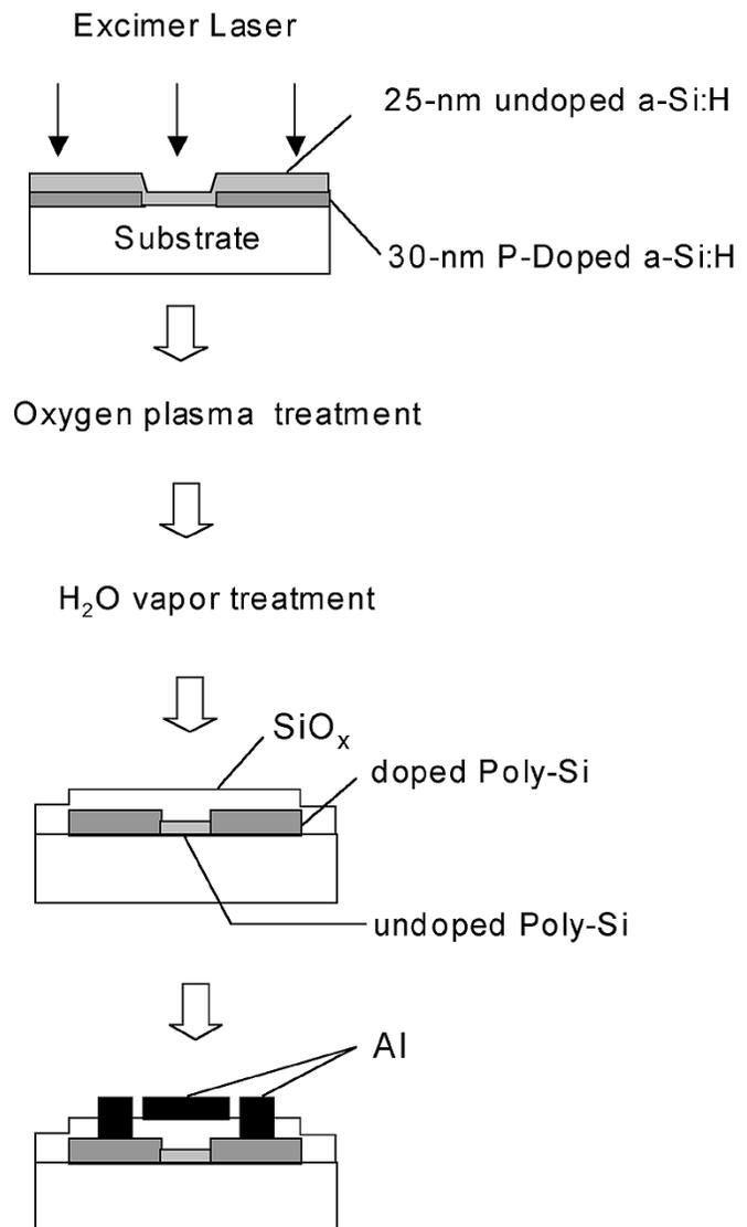
Fig. 1. Schematic process steps for fabrication of poly-Si TFTs.
