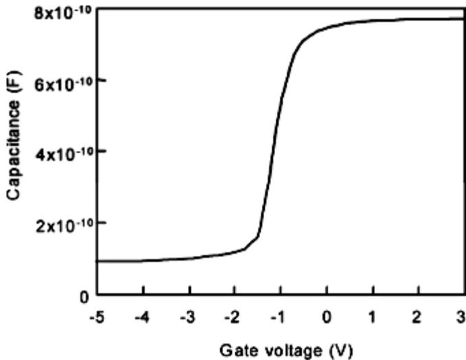
Fig. 2. Capacitance vs voltage characteristics with high frequency at 1 MHz for Al-gate MOS capacitors with 120-nm-thick  $\text{SiO}_x$  films for n-type substrates fabricated by thermal evaporation of  $\text{SiO}$  powders at room temperature in oxygen radical. The area of the Al electrodes is  $0.01 \text{ cm}^2$ .
