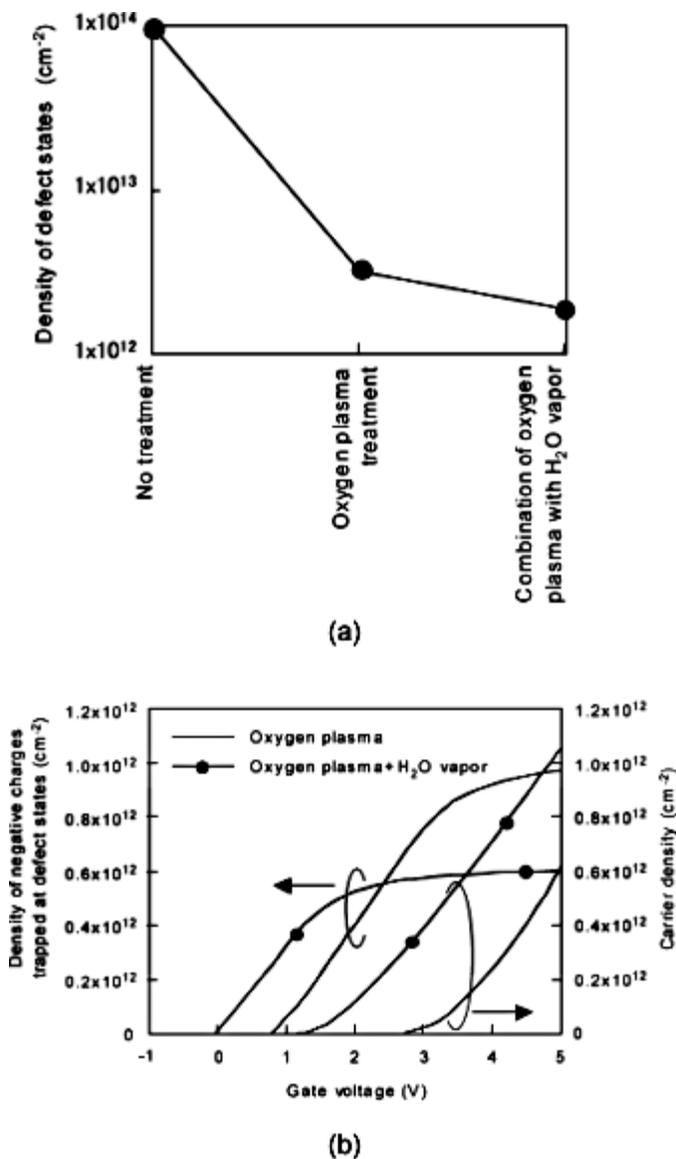
Fig. 4. (a) Change in the density of unoccupied defect states in the flat-band condition with defect reduction steps. (b) Calculated electron carrier density and the density of the negative charges trapped at defect states for TFTs fabricated with oxygen plasma treatment and combination of oxygen plasma with high-pressure  $\text{H}_2\text{O}$  vapor heat treatment.
