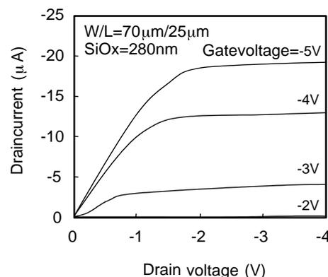
Fig. 4. Output characteristics of p-channel poly-Si TFTs with a channel length of  $25 \mu\text{m}$  and a channel width of  $70 \mu\text{m}$ .
