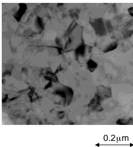
Fig. 2. Micrograph of the bright field image of transmission electron microscope (TEM) plane view for 50-nm-thick silicon films crystallized by the rapid joule heating of metal films at  $140 \text{ V}$ .
