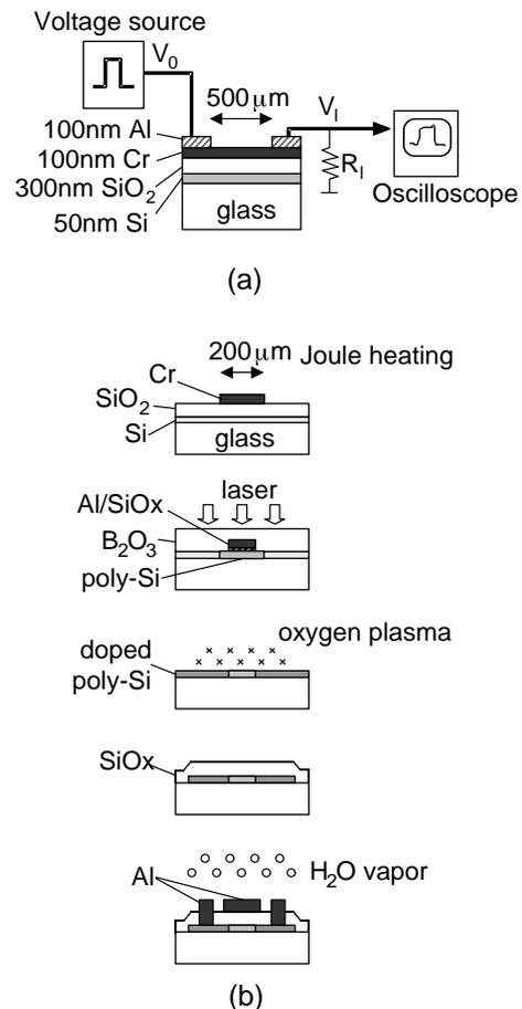
Fig. 1. Schematic apparatus of the rapid joule heating of metal films and the cross section of the layered structure of samples (a). 5-μs-pulsed voltage was applied to 100-nm-thick Cr strip with a length of 500 μm and a width of 200 μm. (b) is schematic fabrication flow of poly-Si TFTs.
