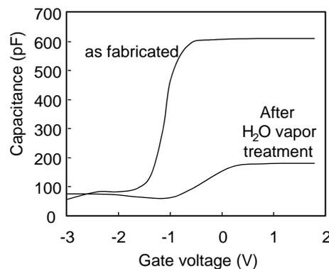
Fig. 3. C-V characteristics at  $1 \text{ MHz}$  for Al gate metal-oxide-semiconductor (MOS) capacitors with  $SiO_x$  as fabricated and treated with  $1.3 \times 10^6 \text{ Pa-H}_2\text{O}$  vapor heating at  $200^\circ\text{C}$  for 3 h. The area of gate Al metal was  $5.5 \times 10^{-3} \text{ cm}^2$ .
