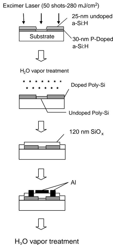
Fig. 1. Schematic fabrication steps of poly-Si TFTs.
