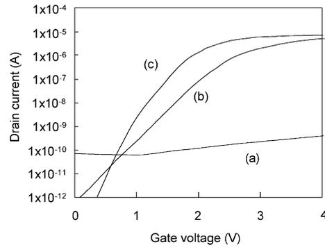
Fig. 3. Transfer characteristics for TFTs fabricated with no H<sub>2</sub>O vapor heat treatment (a), H<sub>2</sub>O vapor heat treatment after laser crystallization (b) and additional H<sub>2</sub>O vapor heat treatment after TFT fabrication (c).
