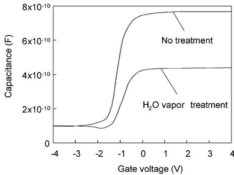
Fig. 2. Capacitance vs voltage characteristics with high frequency at 1 MHz for Al-gate MOS capacitors with 120-nm-thick SiO<sub>x</sub> films for n-type substrates fabricated by thermal evaporation of SiO powders at room temperature in oxygen radicals. The area of the Al electrodes is 0.01 cm<sup>2</sup>. High-pressure H<sub>2</sub>O vapor heat treatment was carried out at 260°C and 1.3 MPa for 3 h.
