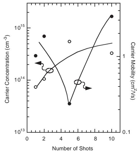
Fig. 4. Carrier concentration and carrier mobility obtained by the Hall effect measurement, with respect to the number of laser shots ( $320 \text{ mJ}/\text{cm}^2$ ).
