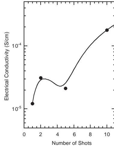
Fig. 3. Variation of electrical conductivity, with respect to the number of laser shots ( $320 \text{ mJ}/\text{cm}^2$ ).
