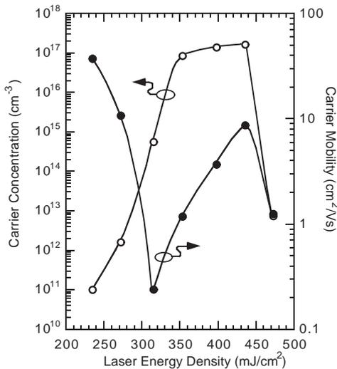
Fig. 2. Carrier concentration and carrier mobility obtained by the Hall effect measurement, with respect to the irradiated laser energy density (step-up irradiation).
