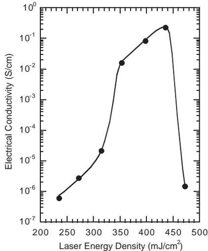
Fig. 1. Variation of electrical conductivity, with respect to the irradiated laser energy density (step-up irradiation).
