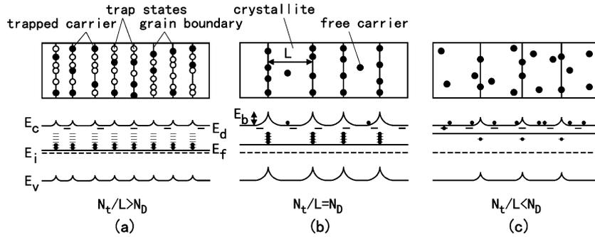
Fig. 5. Schematic diagram of localized-trap-states model and corresponding band structure. Along with increasing laser energy density, the band structure varies from (a) to (c).
